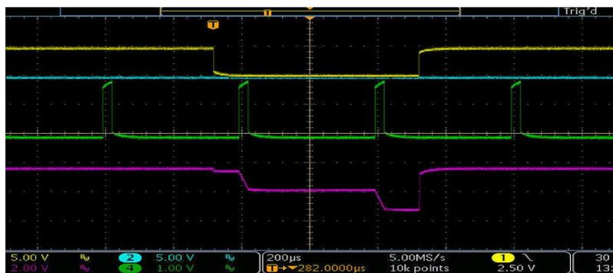
Fig .5Oscilloscope traces: yellow trace is an integrating gate signal; green trace is input pulse; purple trace is output signal.
